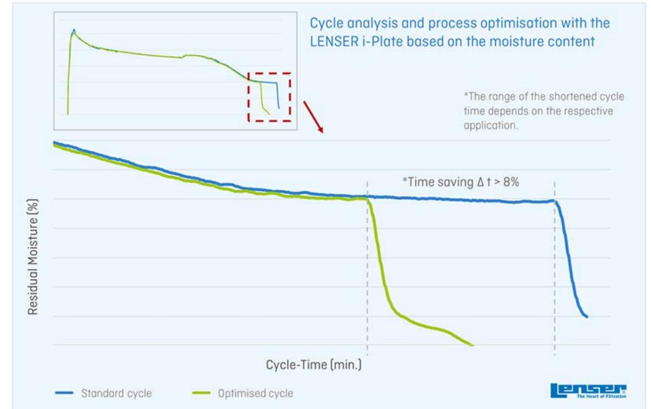
The constant moisture content in the filter cake during the post-pressing process indicates the optimum end of the filtration cycle at an early stage. Ensuring a constant moisture content of the cake at the end of the cycle is important and decisive for subsequent process steps in countless applications. Depending on the application, significant time and energy savings can be achieved.
